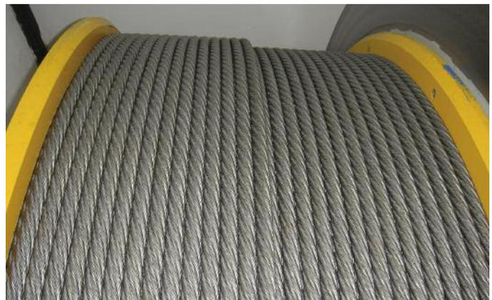
**“Any type of spooling damages rope,” Seidenather says, “But on a Lebus drum, all the damage is in the crossover section [pictured, left] and can be predicted and accounted for.” Perfect spooling, [pictured, right] ensures each coil is supported evenly by two coils below.**
