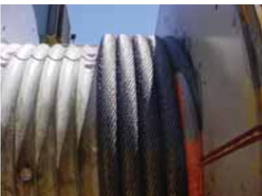
Parallel grooving on a winch drum...
