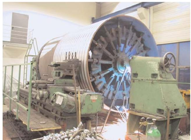
The Braun lathe can make drums up to 4.5 metres diameter
