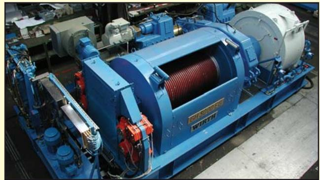
A Wirth GH 3000 draw-works, similar to – but half the power of – the new GH 6000 that is now being developed
