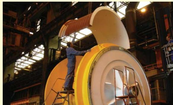
This is the drum of the 405-tonne winch on Total Fina Elf's new Dalia FPSO vessel.
