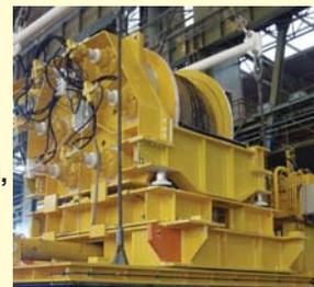
International Engineers GmbH delivered a pair of grooved split drum sleeves. The drum is 2690mm diameter and holds up to five layers of Redaelli 120mm diameter galvanised steel rope, one of the biggest non-rotating wire ropes ever made.
