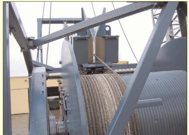
A Lidan Marine launch and recovery system for Remote Operated Vessels (ROVs)
