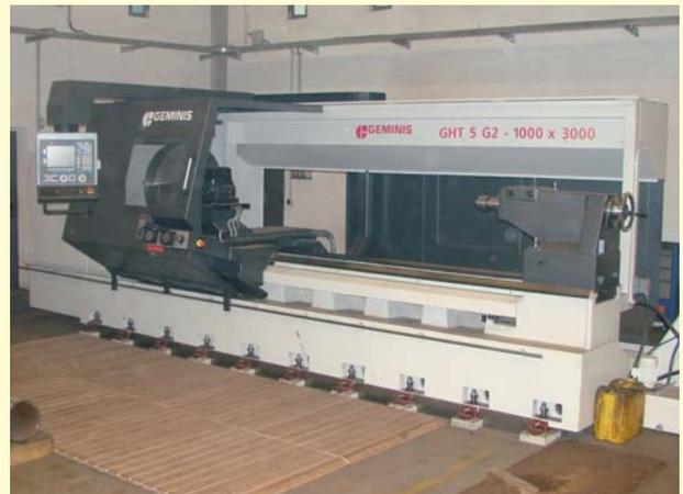
Despite the current difficult economic climate, Lebus continues to reinvest in the business. It has recently installed in its main workshop a new Iberimex-Geminis CNC turning lathe with a special control unit for forming both parallel and helical grooving. It has the capacity to work on tubes up to 1000mm in diameter, 3000mm long and up to 4800kg in weight.
