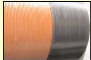
Synthetic rope spooling perfectly, from the bottom layer to the top
